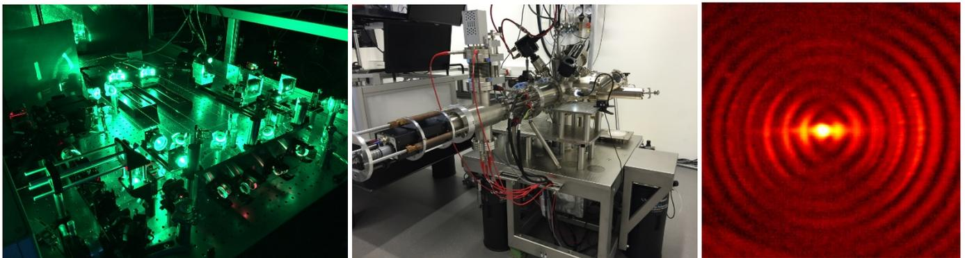
*Left: Dual channel OPCPA system for the generation of two independently tunable ultrashort laser pulses in a pump-probe configuration. Center: PhotoEmission Electron Microscope - PEEM. Right: PEEM-measured electron-photon wavepackets excited by a laser beam incident on a ring-type nanoantenna.*
