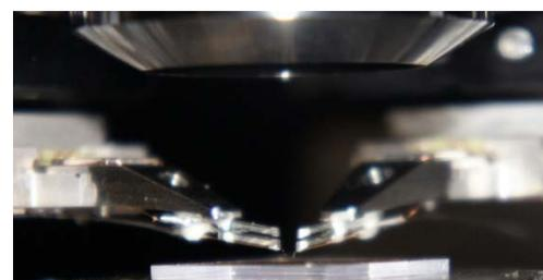
*Left: Schematic for the excitation of a superfocusing surface plasmon-polariton at a metalized fiber tip by resonant coupling to a propagating fiber mode. Right: Two-tip nearfield scanning optical microscope for direct measurement of the optical nearfield Green's function of photonic nanostructures.*
