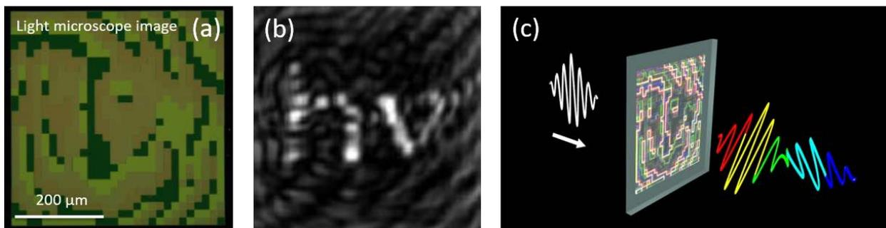
Fig. 1: (a) Light microscope image of a wavefront shaping semiconductor metasurface designed to interact with continuous light waves. (b) Image of the letters *hv* produced behind the metasurface for illumination with an infrared laser. (c) An artist's impression of a photonic metasurface interacting with a femtosecond laser pulse
