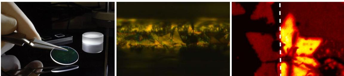
*Left: A monolithic optical cavity loaded with 2D-materials. Center: An optical fiber coated with 2D-materials. Right: Fluorescence of a 2D-material, partially enhanced by underlying nanoresonators.*
