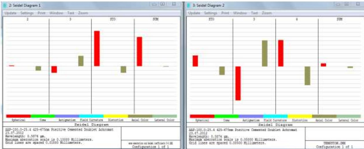
It is seen, that the the system is quite bad for the reversed lens. Therefore the catalog component should be used only with incoming collimated light.
