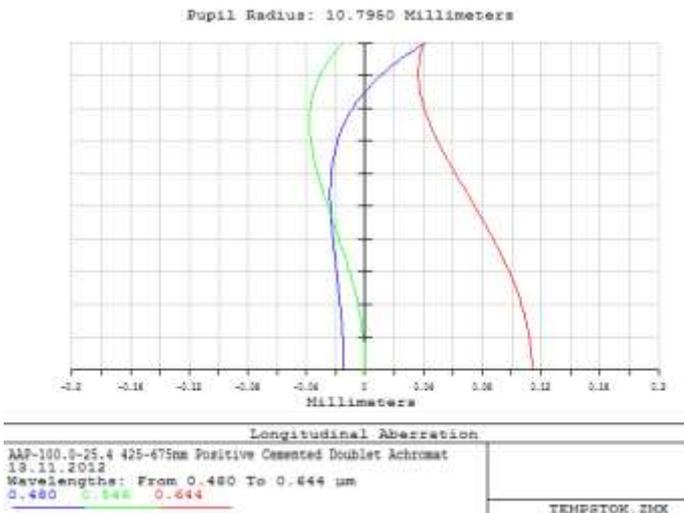
The largest spherical aberration in the green can be obtained by the text output and is  $s' = -0.0377$  mm. this value corresponds to a relative pupil height of 0.76.
