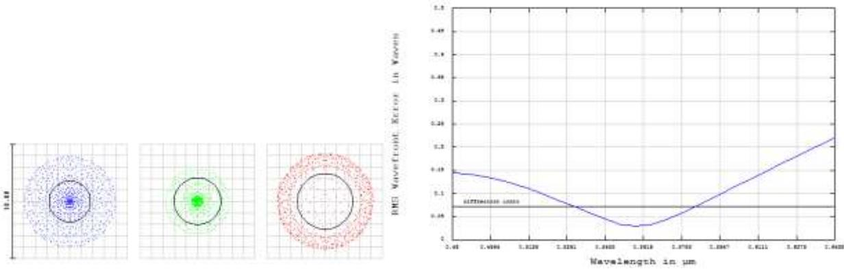
If we now also optimize the three radii of the achromate, we get a diffraction limited performance nearly over the complete spectrum.
