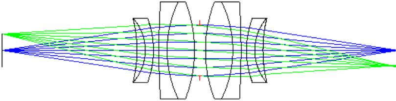
Due to theory, only astigmatism and field curvature are remaining. This can be seen at the Zernike coefficients and the spot diagram, which contains elliptical shapes in the field.
