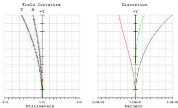
If now the system is kept exact symmetrical and the first group is optimized by radii only it is assumed, that astigmatism and field curvature should be corrected. Thick meniscus lenses and a smaller beam diameter in the middle part solves this requirement best. Exactly this is obtained by numerical optimization. The system is now nearly diffraction limited. The spots show no asymmetrical contribution due to the fact, that the coma is zero.
