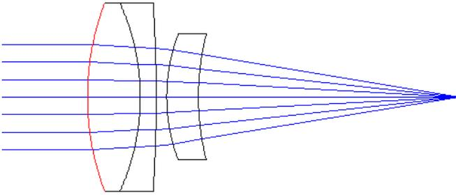
The wavelength combination e F' C' is selected. It is seen, that the system is diffraction limited only near the green line. Spot rms value for the e-line is  $D = 0.858 \mu\text{m}$ .
