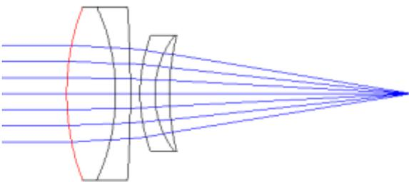
The spot for green now is  $0.799 \mu\text{m}$ , if a quick focus is performed for only green. If all wavelengths are used, the spot is  $1.425 \mu\text{m}$  and the quality is more smooth over the wavelengths. The diffraction limit is not fulfilled for blue and red.
