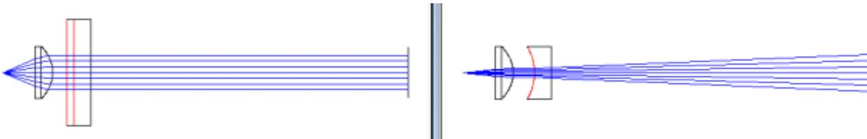
For a Galilean telescope with factor 4, the second lens must have a focal length of  $4 \times 25.1 \text{ mm} = 100.4 \text{ mm}$ . In the same lens catalog one can find the following lens:
