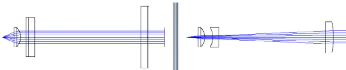
To focus the beam into a fiber with numerical aperture 0.1, the focal length must be not smaller than  $f = 4.32 \text{ mm} / 0.1 = 43.2 \text{ mm}$ . A lens of approximately this size can be found in the catalog of Melles Griot as an achromate. This helps in getting a better correction: LAO-44.0-14.0
