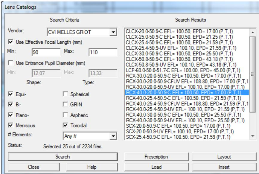
The lens is inserted, turned around to get a better performance and also tilted by  $90^\circ$  in the azimuth. A first guess gives a distance of  $100-25=75$  mm between the telescope lenses to get a collimated x-section. But from the spot diagram with direction cosine option it is seen, that the angle distribution is not equal in both sections. Due to the finite positions of the principal planes of the lenses, the distance must be optimized with an angle criterion default merit function.
