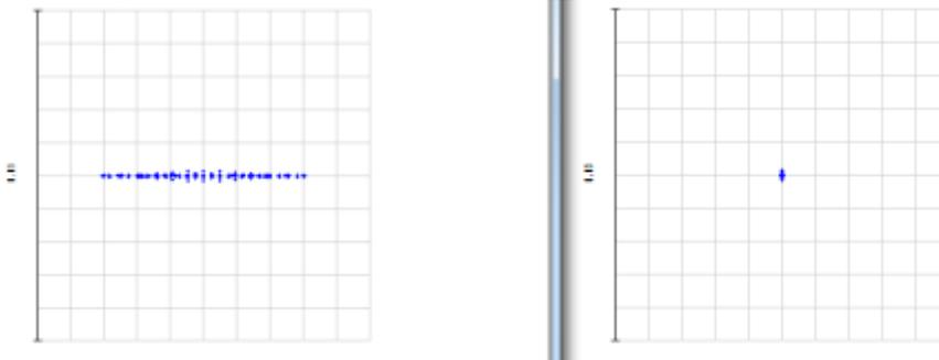
The footprint diagram now shows a rather circular cross section. The residual error can be neglected and comes from the fact, that for this wavelength, the catalog focal lengths are not exact.
