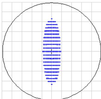
In the next step, a Galilean telescope with factor  $\Gamma = 4$  must be found to enlarge the diameter of the x-section to the same value as in the y-section. First a negative cylindrical lens with a rather short focal length must be found.
