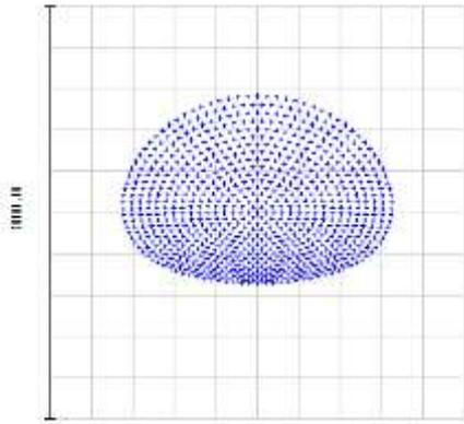
Since the spherical mirrors induce a large astigmatism, the focussing only looks fine in the y-z-plane. The elliptical shape near the circle of least confusion dominates over the coma.
