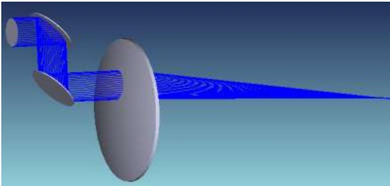
Footprint: the size of the beam in the local system is  $D_x = 20$  mm,  $D_y = 28.3$  mm
