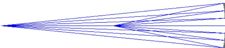
c) An additional surface is introduced after the object and a coordinate break is defined with 60° tilt around the x-axis.
