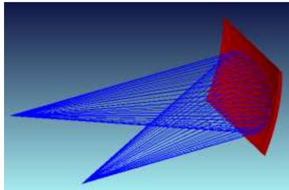
If the ray trace is calculated for the central ray, we get the incidence angle  $13.90^\circ$ . Therefore the bending of the central ray is  $27.8^\circ$ .
