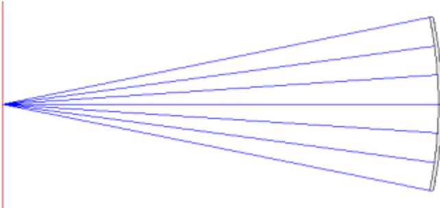
b) Image distance doubled and a simple merit function (default) is used to optimize the radius  $r$  and conic constant
